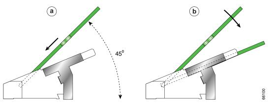
Step 9 Gently press the SODIMM down using your index fingers, distributing even pressure across the module until it locks into the tabs. (See Figure 56b.)
